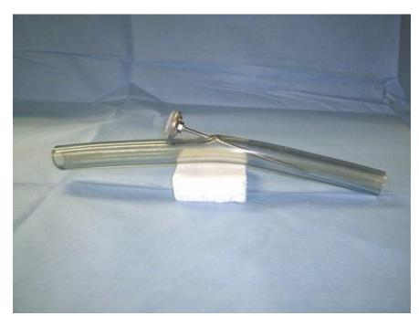
This picture shows a simple method using an inexpensive rapid read thermometer to measure water flowing in a hose (in this case milker line hose). The left hand end of the hose attaches to the water mixer faucet a sink.
