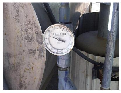
a remote sensor. In this case the sensor is in a tank holding milk that is being heated for feeding to calves. Close examination shows that the current temperature is approximately 90° F.
